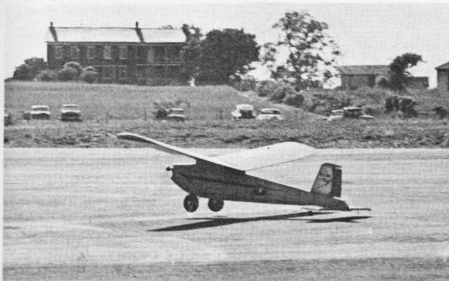
Touch-down of "Multi-Bug" on a touch-and-go landing. Note wheels and skid are all 2" above ground and elevator is almost full up. Shows what dual proportional can do.
