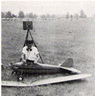
Left: Joe Raspanti ground-tests his Super Buccaneer, second at the 1939 Nats. Note the tripod-mounted control box. Center: His control box used a telephone dial. Rudder and engine controls were dialed in. Right: The four-tube receiver and sensitive relay inside the cabin.
