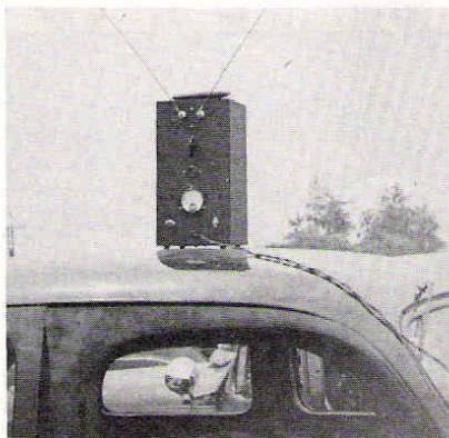
Left: Bieberman's transmitter with "V" antenna sits on top of his car at the 1939 Nats. Right: Bieberman's one-tube receiver is seen here through the transparent panel in the fuselage.
