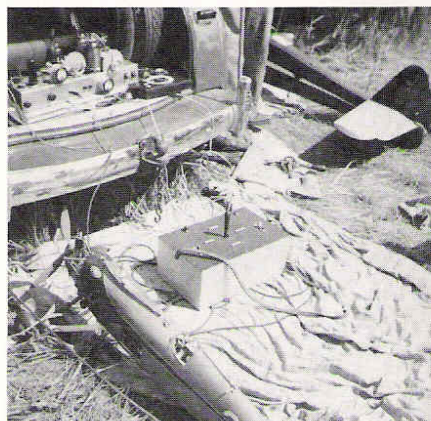
Left: Winnie Davis launches Siggy's 14-lb. RC plane. Right: Siegfried's 50-watt transmitter can be seen sitting in the car trunk, control console on the ground, tail of the 14-footer in the background. Plane in the foreground is a backup. Siegfried went on to finish in third place.
