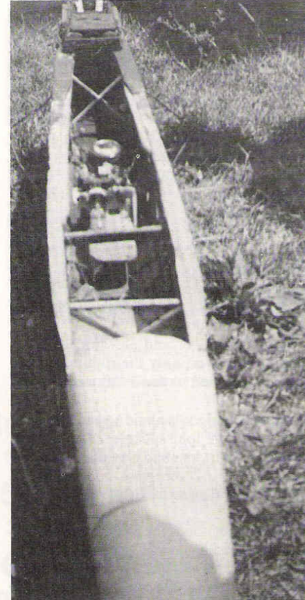
Wasman's fuselage carried an RK-62 one-tube receiver and escapement rudder. It didn't make a successful 1939 Nats flight.
