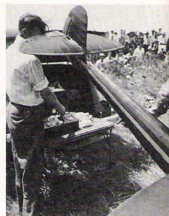
Left: Earle's 9 1/2-ft. original with REM and three receivers. Right: Earle holds the plane while a friend works the control box on the table. Transmitter located in the car's trunk.
