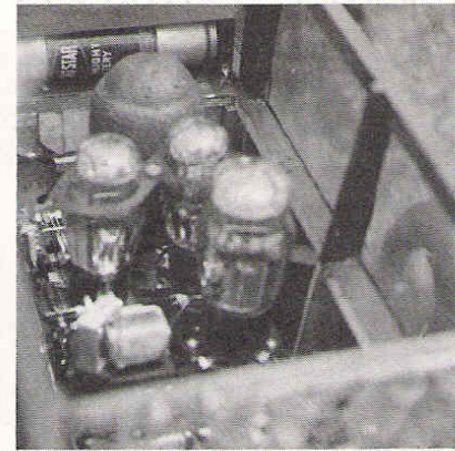
Left: Joe Raspanti ground-tests his Super Buccaneer, second at the 1939 Nats. Note the tripod-mounted control box. Center: His control box used a telephone dial. Rudder and engine controls were dialed in. Right: The four-tube receiver and sensitive relay inside the cabin.
