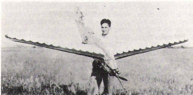
Left: Elmer Wasman holds his 10-lb. RC model which won third place in 1937. It had rudder/aileron and elevator control, also engine cutoff. Right: Rear view of Wasman's plane shows the air-driven four-bladed propeller mounted on front of the fin for power for moving the control surfaces. Photos from Wasman. Below: Jacksonville, FL paper clipping (1937) shows Wasman explaining his White Mystery to students.
