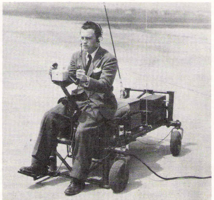
Left: Leo Weiss (arm in front of the rudder) working on a Denny Radio-Plane at Wright Field in 1939. Right: Ground control unit used to control Culver Cadets and larger RC drones. The GCU also carried communications gear. Leo is shown at the controls of his 1939 design. Below: Oops! Even professional RCers sometimes make a “hard” landing, as we see in this picture of a poor Culver Cadet at Wright Field in 1939.
