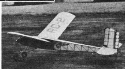
Ancient-looking German design, like most of its kin, fitted with two-speed engine, rudder and elevator controls.
