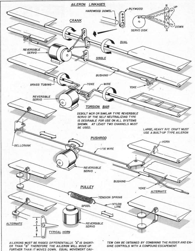
SES A YAWING ACTION OPPOSITE TO THE DESIRED TURN. THIS IS CAUSED BY THE MORE PRONOUNCED DRAG OF THE DROOPING AILERON.
