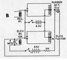
pulse speeds, up to about 5 PPS. Therefore, the length of time the elevator is held to either extreme position depends solely upon the rudder pulsing rate.
