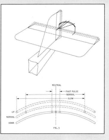
Galloping Ghost, simply stated, is utilizing a single tone from a transmitter in such a fashion as to provide information to operate rudder, elevator, and motor from one mechanical actuator.
