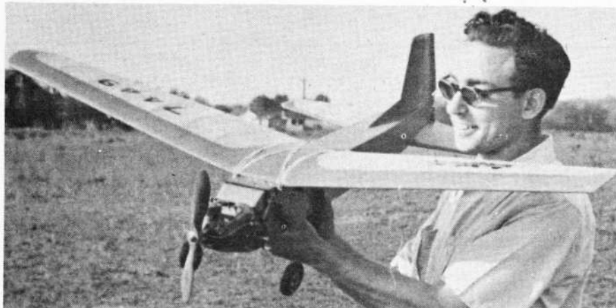
Phil Greenberg's Jasco R/C Master uses an E.C.C. receiver and a Super Aerotrol escapement. The sponge-mounted nose section effectively eliminates vibration effects of the engine.
