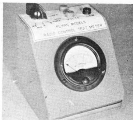
Above: The completed FM Multimeter, used to check all components of your R/C equipment.
