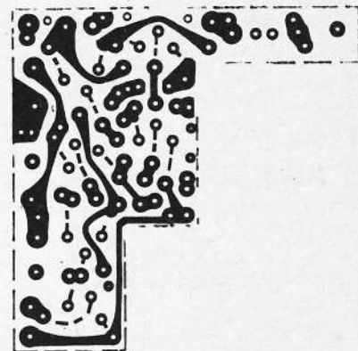
Above—Conductor side of servo/discriminator printed circuit board. (Actual size)
