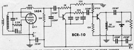
NOTE: MAKER SUGGESTS USE OF AMPEREX 6007 TUBE IN PLACE OF 1AG4; NO OTHER CHANGES NEEDED. 13 MA. FILAMENT DRAIN IS MAIN ADVANTAGE
