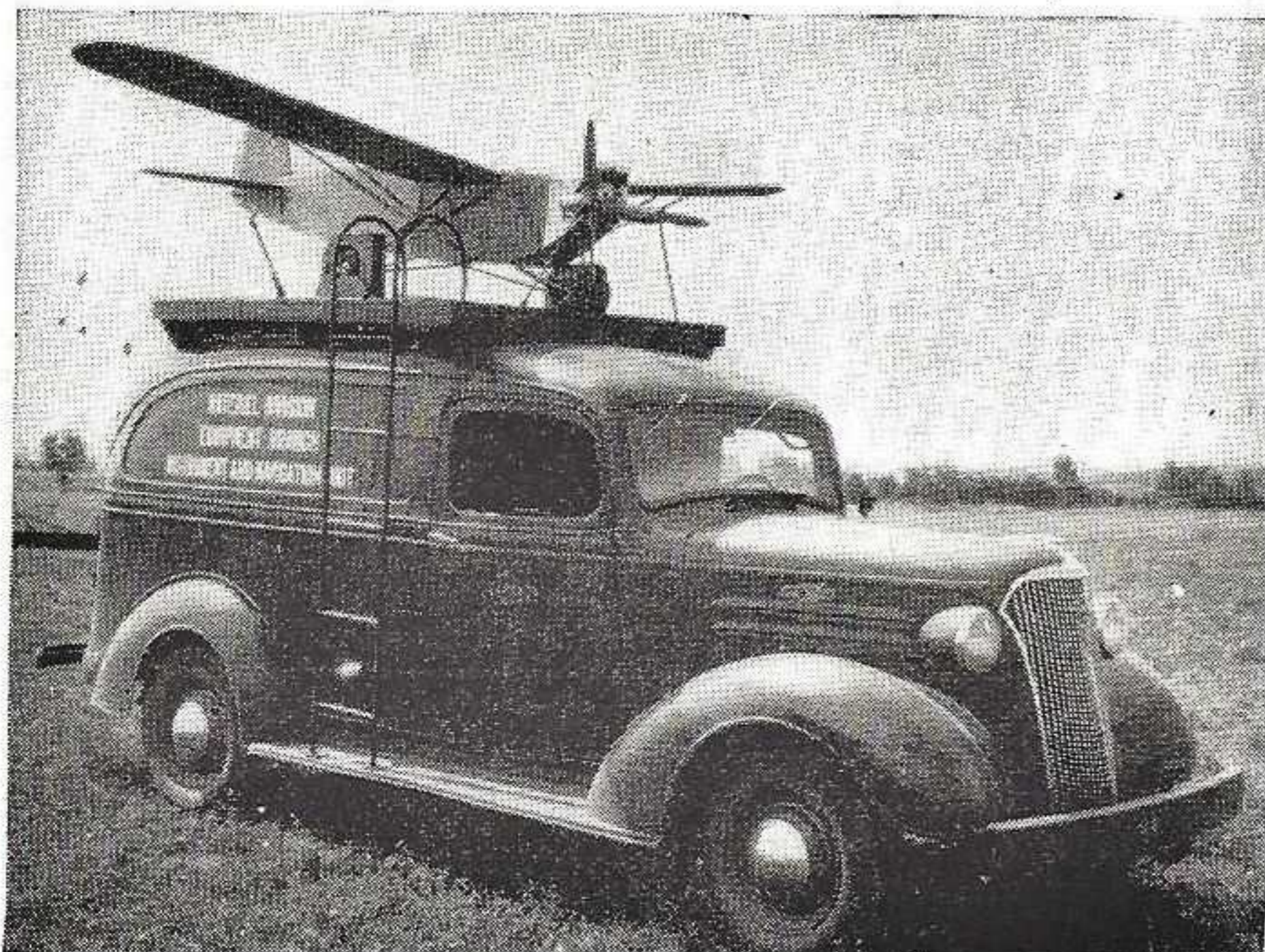
The aerial target plane is transported from place to place securely mounted on top of the control car, as shown
