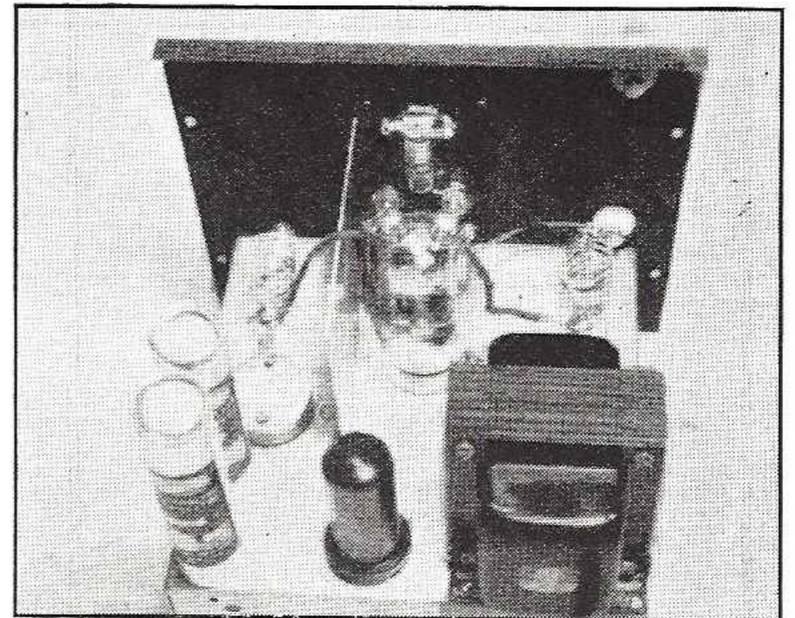
Fig. No. 8. RK34 with oscillator and amplifier coil
