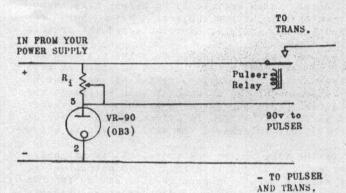
In looking in Vol. 1 #4, I noticed an answer on 3V4 They recommend use of batteries, pulser on power supply. not so, unless you like to buy them. My transmitter has operated a lot of days, four to five hours at a time, without a skip. The following may be of use to others, being easy and inexpensive to use, the VR-90 (0B3) is reliable.
