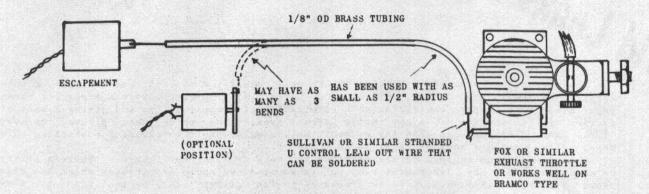
This hookup will work with an escapement on 1/8" rubber or a servo. Has been tried with Bonner Single SN Escapement and DeBolt 3r3na.
