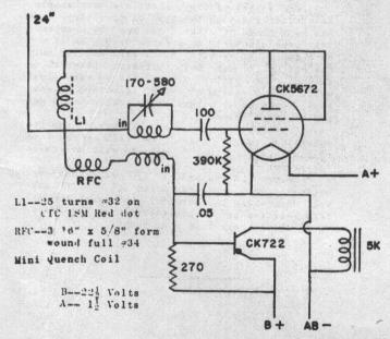
many hard tubers. The circuit features an extremely low idle through the relay which goes up to about 5 mils. upon receipt of signal. As mentioned in the original article where the sensitivity is lacking the rf choke may need to be changed, many go to a higher inductance, although many people write us that they have had to make no changes whatever.
