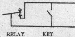
PULSER RELAY IS WIRED ACROSS KEY SO THAT PULSER ACTS AS AUTOMATIC THUMB
