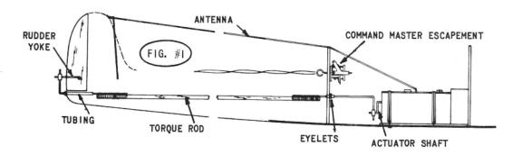
Figure #1 shows plywood floor cemented directly to bottom of fuselage. Cut % x % hole for on-off switch thru floor and bottom of fuselage. Switch is at rear of hole which allows clearance for forward movement, protecting switch in the event of hard impact. Figure #2 shows raised floor if Receiving Unit cannot be mounted to bottom of fuselage. In this case, blocks are installed to raise floor to desired height.
