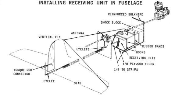
Place Receiving Unit in fuselage so that your model balances at the point designated on its plans. If no balance point is available, then balance model ½ back from front of wing with all equipment in place and model assembled.
