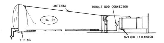
Torque rod is made from 1/4" sq. hard Balsa. Ends are 1/16 Music wire. Bind and cement in place, leaving wire straight. Drill hole slightly larger than tubing, and insert tubing (at least 1" long) thru back of fuselage as shown. Do not cement in place yet. Tubing should fit wire snugly — yet freely.
