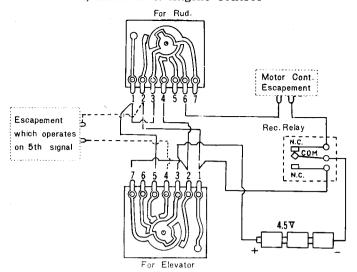
With two Compound Escapements in shown wiring, upper & lower ones can be operated for Rudder & Elevator Control respectively. It is economical because there is no current on Rud Escapement while Elevator Escapement is in operation.
