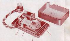
Remove the lid after unscrewing the nut at the bottom of the lid. After removing screw A the contact set B can be lifted approx. 1/4 – 3/8". Attention: do NOT bend the contacts! Using one of the two small recesses C the steering disc E can be lifted with a small screw driver and removed from its support.
