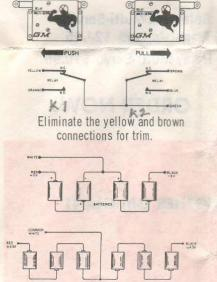
RELAY SERVO: The G.M. Geni may be used as either self-neutralizing or trim. The drawing below (left) shows the proper way to hook up the Geni for the self-neutralizing mode of operation. To use the unit as a trim servo, merely omit the yellow and brown connections and stow these wires.
