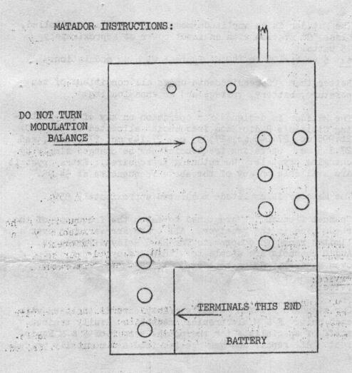
CAUTION: OBSERVE BATTERY POLARITY. SERIOUS DAMAGE WILL RESULT FROM REVERSED VOLTAGE.
