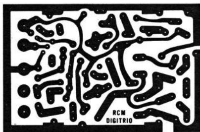
Decoder PC board shown three times full size. Actual size PC board shown at left. Either can be used for photographically reproducing the circuit board.
