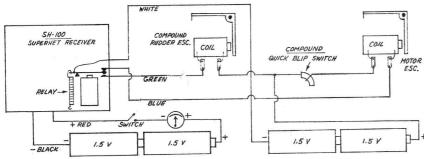
Voltage measurements taken with Heathkit lM-13, V.T.V.M. 5 volt, minus DC scale. Common lead to plus 3 volts receiver battery. Receiver idling, No signal from transmitter. Note divided circles on diagram, top no voltage measured, lower No is circuit board hole that identifies copper land to which place DC probe. Normal measurement can vary plus or minus 20% due to component tolerances.
