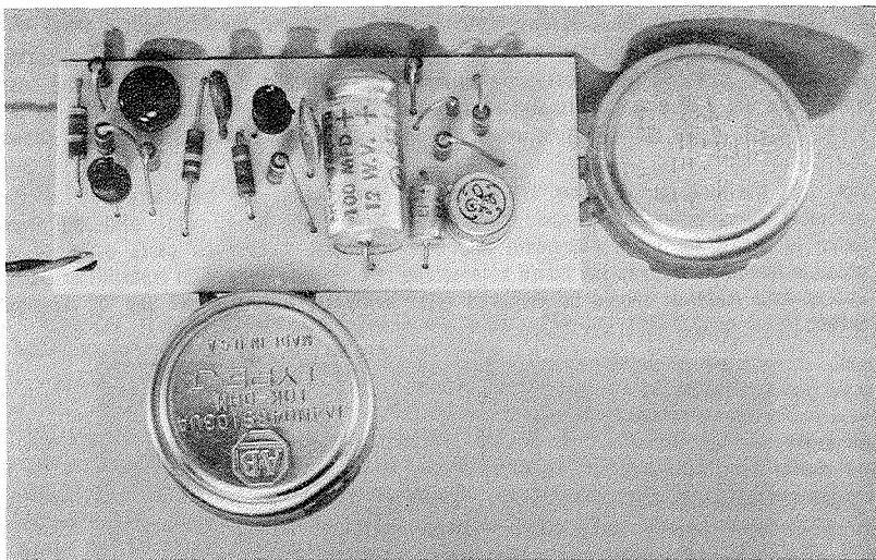
PHOTO 2A-Top view of conversion kit P.C. Board with all components in place; this photo matches Fig. 3.
