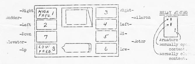
The relays should be connected as shown in the above diagram to conform to the nomenclature on the control stick and switches on the transmitter.
