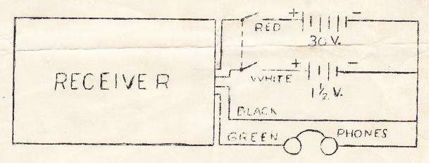
A plug and socket are provided for insertion between the set and batteries for easy removability of the set.
