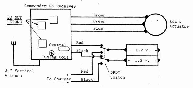
After you have installed your receiver, leave the transmitter antenna collapsed and move away from the transmitter, observing the pulsing action. If pulsing quits, stop moving and tune the core in the antenna coil just a slight bit in one direction or the other until pulsing begins again. If you fail to get pulsing after you have turned a half turn on the slug in either direction, move back in closer to the transmitter again. Touch up this tuning until you have range of approximately 100 feet.
