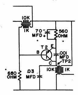
For warm weather use, re-install the  $4.7 \, \mathrm{K}$  and short out the  $70 \, \mathrm{mf}$  -  $560 \, \mathrm{ohm}$  combination.
