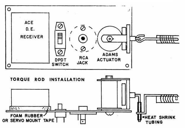
maple bearers mounted on each side of the fuselage, the tray may also be mounted by using double sided servo tape.
