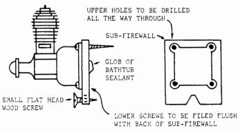
Here is a mounting idea for a Cox .020 Pee Wee in small planes. The unit as shown can be slipped down into place on flat head wood screws. The upper screws can then be tightened into regular firewall to obtain amount of side thrust desired. Size of glob determines amount of downthrust. I use wood screws for everything. The idea is quite simple to make. The engine can be removed in less than a minute for cleaning etc. I have used this same setup on several small models with great success.
