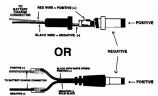
figure, making sure you maintain proper polarity when soldering these connections. Heat shrink tubing is provided to insulate the solder connections.
