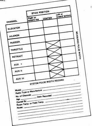
Connect the Datamaster to the elevator channel of the receiver, turn on both transmitter and receiver battery pack. Write down the number appearing in the display in the block marked "center". Move the elevator stick on the transmitter to both extremes recording both blocks for elevator. Then the remainder of the channels can be logged the same way. Now turn off all power again.
