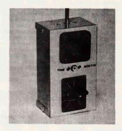
Here is a combination field strength meter and tone monitor. Meter used is 500 ua type and FSM monitor is tunable from frequency ranges of 25 to 54 megacycles.
