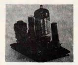
MClOOT--tube and transistor tone receiver at 1000 cycles per second uses 12 volts A and 30 volts B. Features a current rise, has only a 13 mil filament drain, comes completely assembled. Must be used with a transmitter capable of 100% modulation at 1000 cycles per second such as the MC25OT. \$20.95
