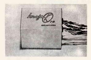
The Kraft Multi-Fli superregen relay-less receiver is housed in a case  $2\frac{1}{2}$ " x 1 7/8" and is only 1 7/8" thick. It is designed to be used with the Transmite servos. It is available only with a 10 channel reed bank but may be used for any number of channels from two on up to ten if desired at any stage of the game. Relay versions also will be available at a little later date.
