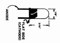
The lens is red and diffused--produces red visible light. Excellent on to off contrast.
