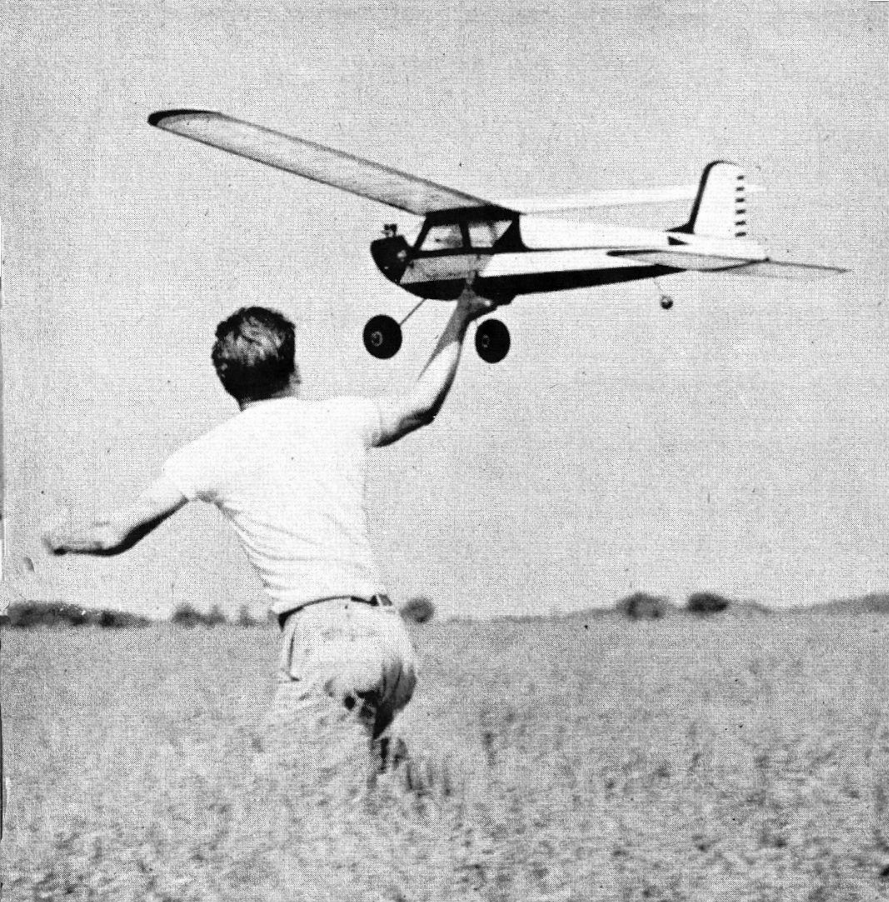
A Rudder Bug gets away. With the compound escapement power approaches, loops are possible.
