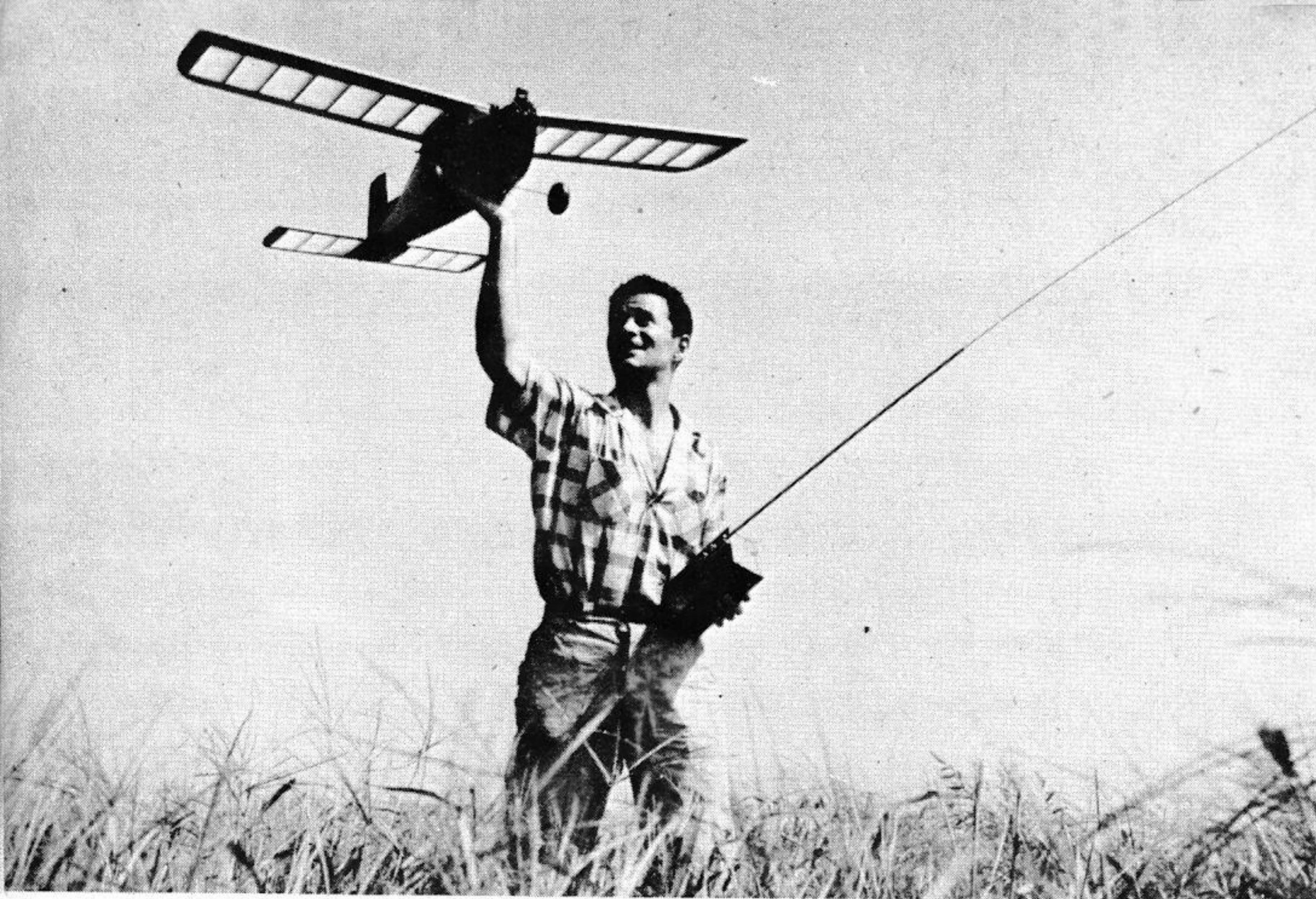
Small size of the plane makes it easy to launch while holding a transmitter. This particular ship was equipped with an Aerotrol, though designed for McNabb, others, as well. Bernie Spira makes the launch.
