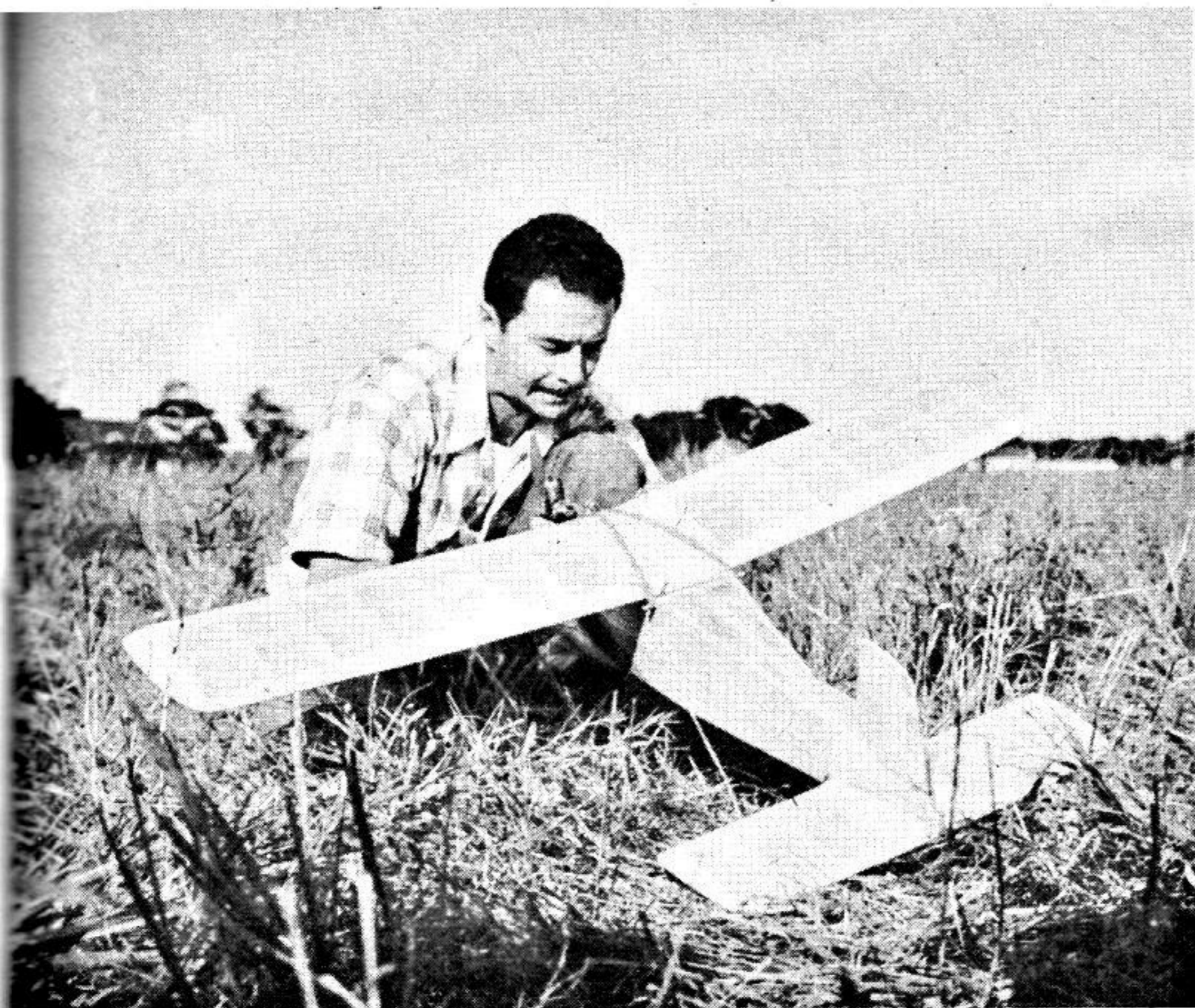
Single-spar wing is knock-off in crash, ties on with rubber looped over two rear, one front, dowels. Stabilizer detachable, ties in place under fuselage. Team racer gear.
