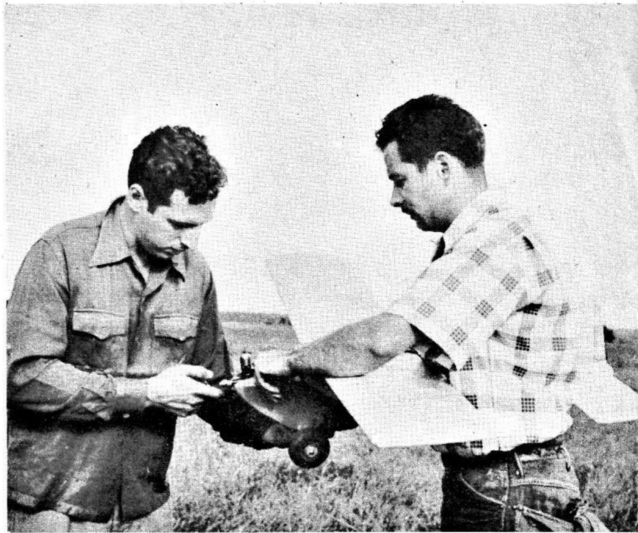
Starting an .08 Mills version. Test job flew well with McCoy 9 and an 8 x 6 propeller. Deep nose and a short gear combine to save props; "few flip overs." Fuse is sheeted.
