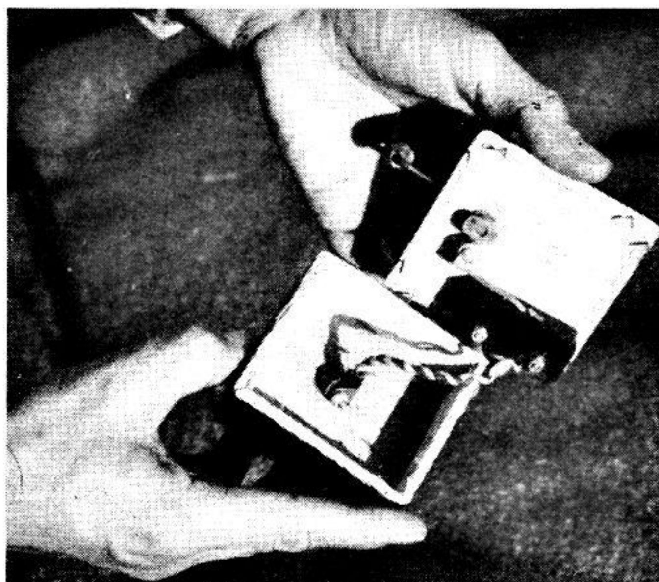
Above—Opened box displays simple mechanism. Cam on stick shaft, riding against roller, closes switch. The box fits in hand.
