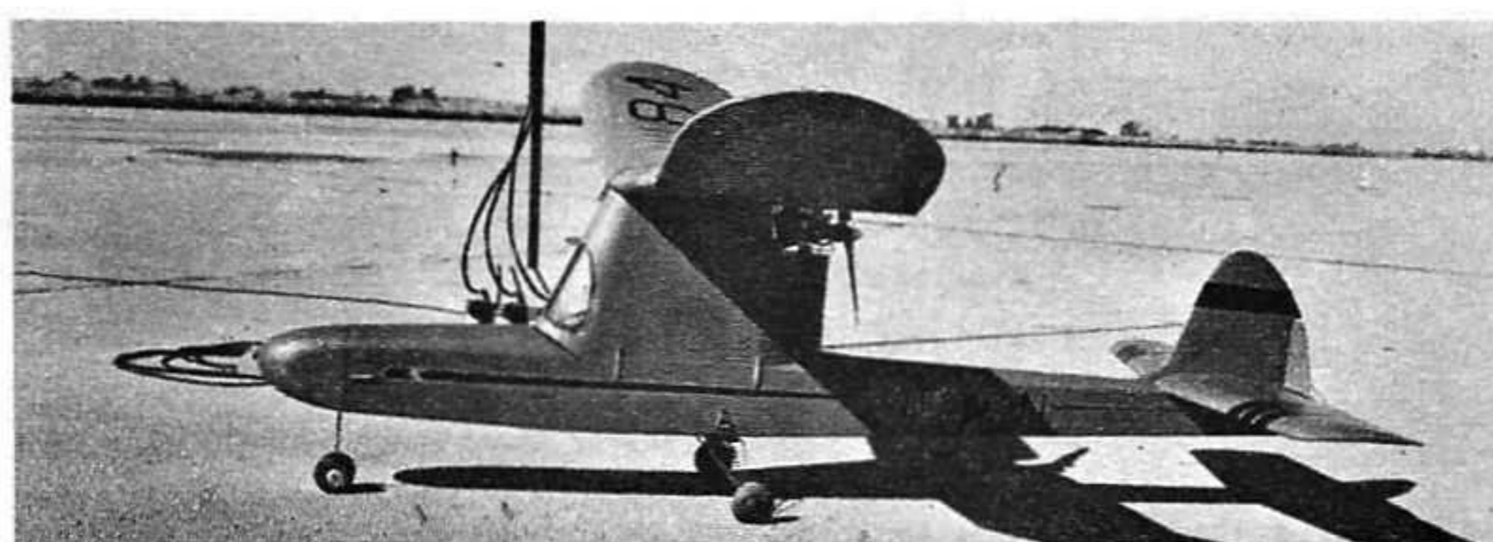
Large pylon is necessary to give clearance since the prop is 20" in diameter
